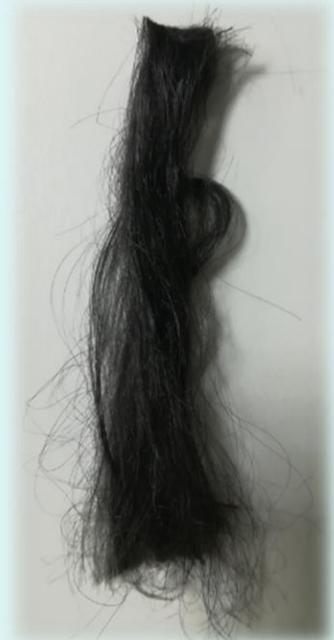
Image of filaments produced with recycled PET waste.
