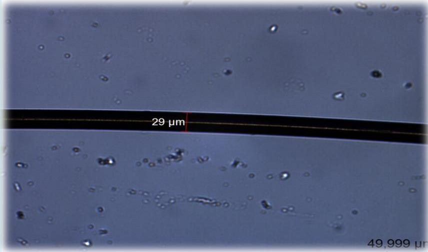
Microscopic image of a filament produced from recycled PET waste.
