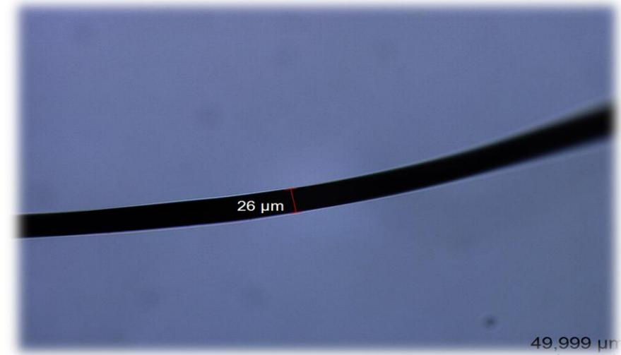
Microscopic image of a filament removed from the original PET textile waste.
