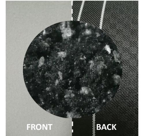
Use of liquid nitrogen in waste in order to keep it below its  $T_g$ , temperature below which the polymer loses molecular mobility becoming more rigid.
