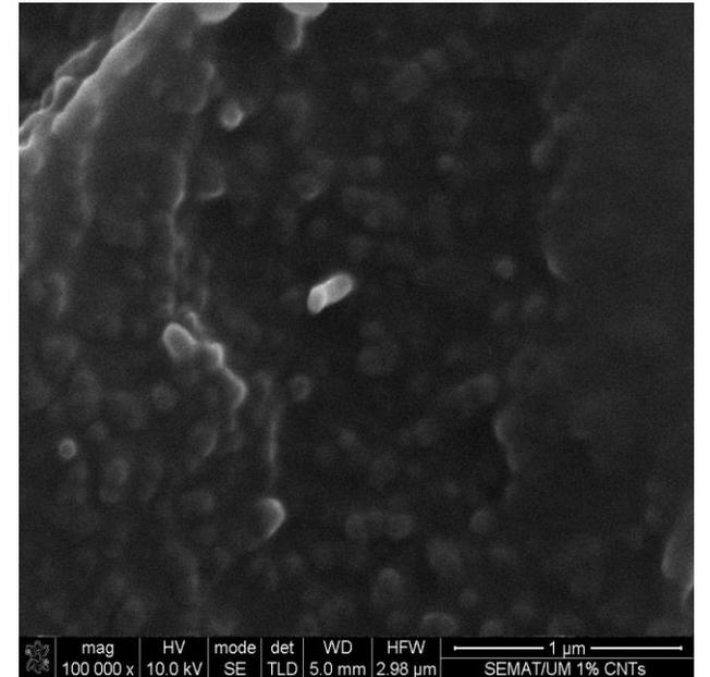
Cross section of the PET40\_rPET60\_1CNT's sample.
